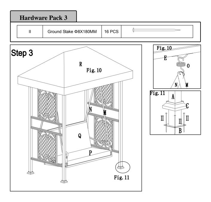
**Fig.10:** Hang the assembled Seat to Middle Cross Beam (E) with Support Hook (O). Put Seat Cushion (P), Back Cushion (Q) on the Seat and place Canopy (R) onto top.
