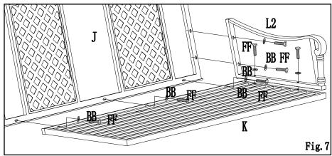
**Step 7**: Connect Back Panel (J), Seat Panel (K), Left Arm (L2) and Right Arm (L1) with Bolts (FF) and Flat Washers (BB). (Fig.7)
