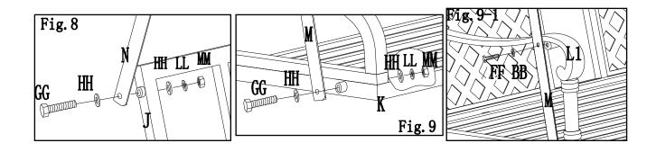
Fig.8: Lock Short Suspender (N) onto Back Panel (J) by using Bolt (GG), Flat Washer (HH), Spring Washer (LL) and Nut (MM). (Fig.8)
