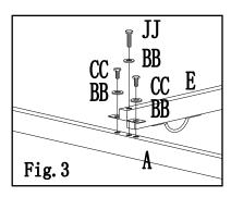
Step 1: Attach Base Cover (C) to Post of Side Panel (A).
